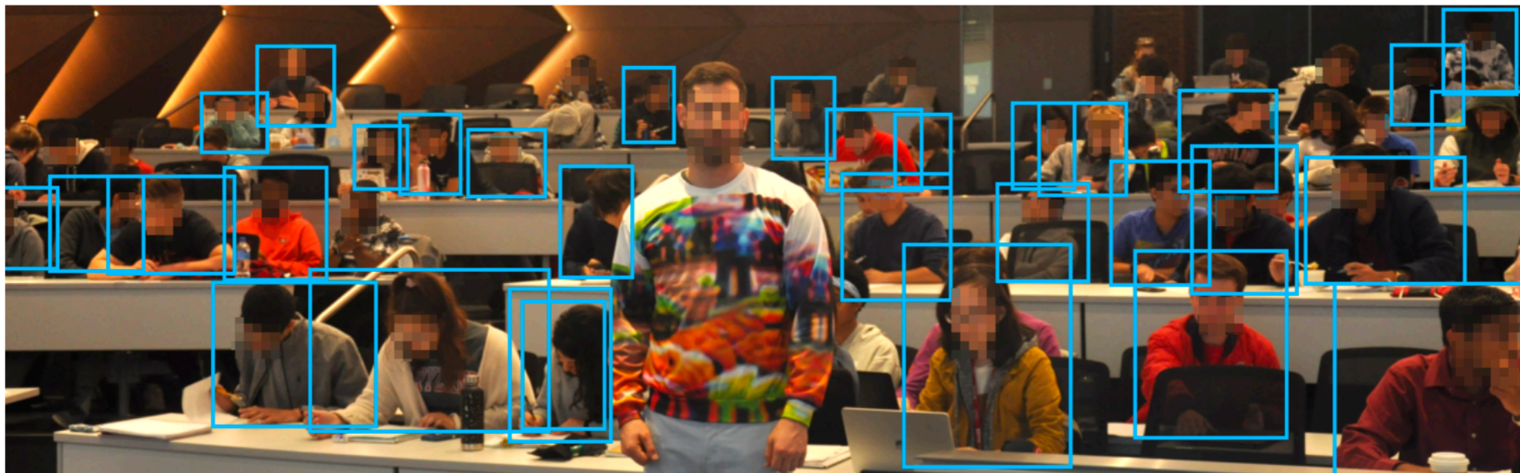
Figure 1: This stylish pullover is a great way to stay warm this winter, whether in the office or on-the-go. It features a stay-dry microfleece lining, a modern fit, and adversarial patterns that evade most common object detectors. In this demonstration, the YOLOv2 detector is evaded using a pattern trained on the COCO dataset with a carefully constructed objective.
